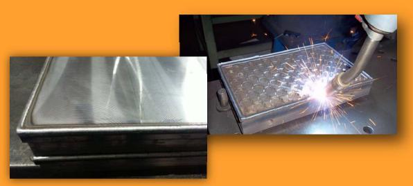
SEAMLESS Cored Wires for Hardfacing of Mould & Punches for Ceramic Tiles
