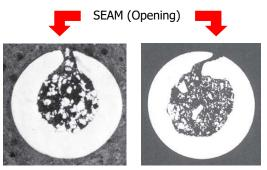
Conventional FOLDED wire has a SEAM This causes MOISTURE ABSORPTION
