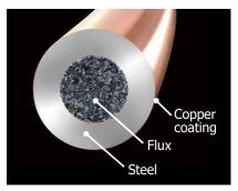
SEAMLESS wire has NO SEAM This means NO MOISTURE ABSORPTION
