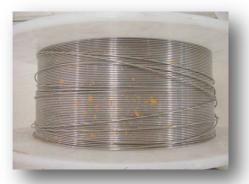
Conventional FOLDED is not Copper Coated—RUST on the surface
